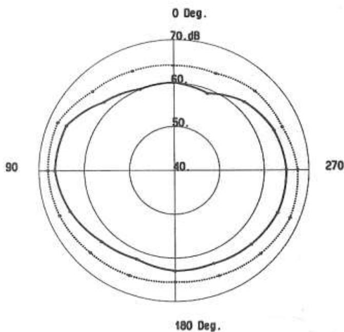
Figure 62 - Sound radiation diagrams of the calling song of a male of *Tympanistalna gastrica*, measured with a 63 Hz high-pass filter (dotted line) and a 1/3 octave band-pass filter centred at 13 kHz (solid line), frequency corresponding to the peak of the calling song spectrum. The measuring microphone was moved along a horizontal plane around the singing male (dB values relative to 20 microPascal).
