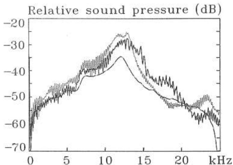
Figure 67 - Effect of reducing the volume of the anterior internal chamber on the spectra of the soft sound pulses. Initial condition - solid line; spectrum after the injection of some vaseline into the chamber - dotted line; spectrum when approximately 3/4 of the anterior chamber was filled up - dash-dotted line
